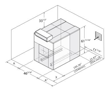
If  $A=47^{1/4}$ " (side burner side door open),  $A'=47^{1/4}$ " (side burner door open): dimensions to be adopted according to the space required for the burner when the door is open.
