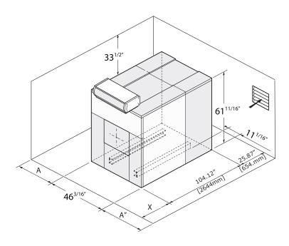
If  $A=47^{1/4}$ " (side burner side door open),  $A'=47^{1/4}$ " (side burner door open): dimensions to be adopted according to the space required for the burner when the door is open.
