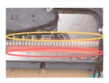
Caution: The numbers indicated on the opposite side (Indicated in red in the above picture) of the terminal strip do not match the wire numbers on the plug harness and should NOT be referenced when making the wiring connection from the harness to the terminal strip.
