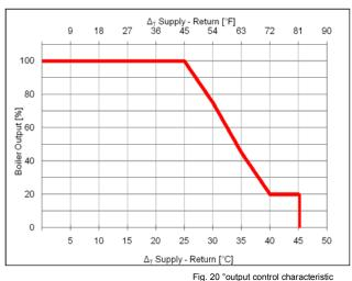
In all cases, modulation is based on the required flow temperature and there is a  $\Delta_T$  dependent output control with the following characteristic. Up to a  $\Delta_T$  of 45°F [25°C] (factory setting, parameter  $\underline{H}$ ) the boiler operates at full output. Between  $\Delta_T$  full load and  $\Delta_T$  part load the output reduces in linear fashion (see fig. 20).
