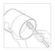
Fig. 29 non return valve being cleaned with soft brush
