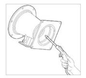
Fig. 30 Venturi being cleaned with compressed air
