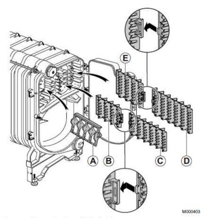
▶Put the baffles in place. Align the convection accelerators with the first fins.
